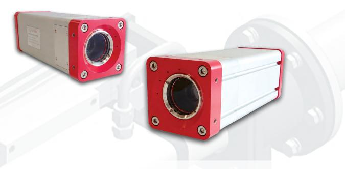
TempVision's two-color spectrum imaging technology measures furnace temperature within its viewing window with a better than 1% accuracy. TempVision simultaneously monitors the temperature and automatically compensates for emissivity variation caused by the soot around the target area. This is a critical capability for precise temperature measurement in a coal-fired furnace environment.
